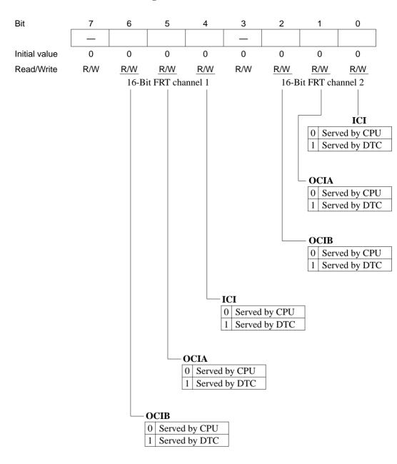
DTEC—Data Transfer Enable Register C
