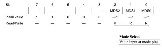
\* Initialized according to the inputs at pins MD2, MD1, and MD0.
