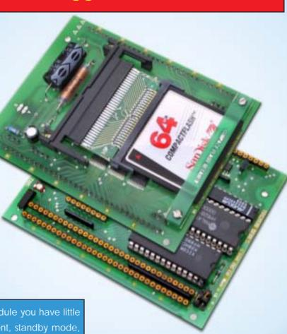
As a Data Logger Module you have little to add to its low current, standby mode, over a gigabyte of memory, 10-bit 8-channel A to D and real-time clock. There are keyboard, graphics LCD, CAN and serial port interfaces. Use Industry standard digital camera Compact Flash and PCMCIA-ATA cards. You can also log to a flash chip on the computer.
